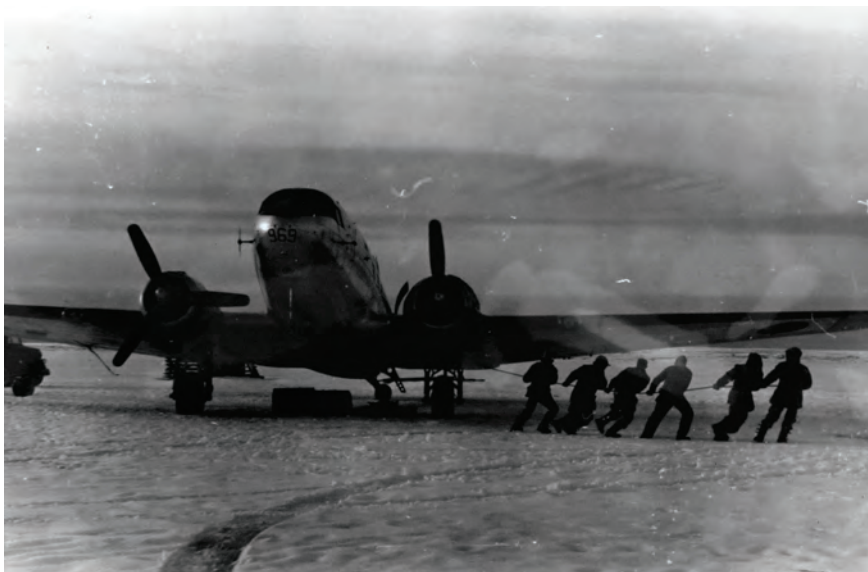
Figure 6-18: Starting the aircraft engine with a rope at Coral Harbour. Source: DHH 181.003 D2261
