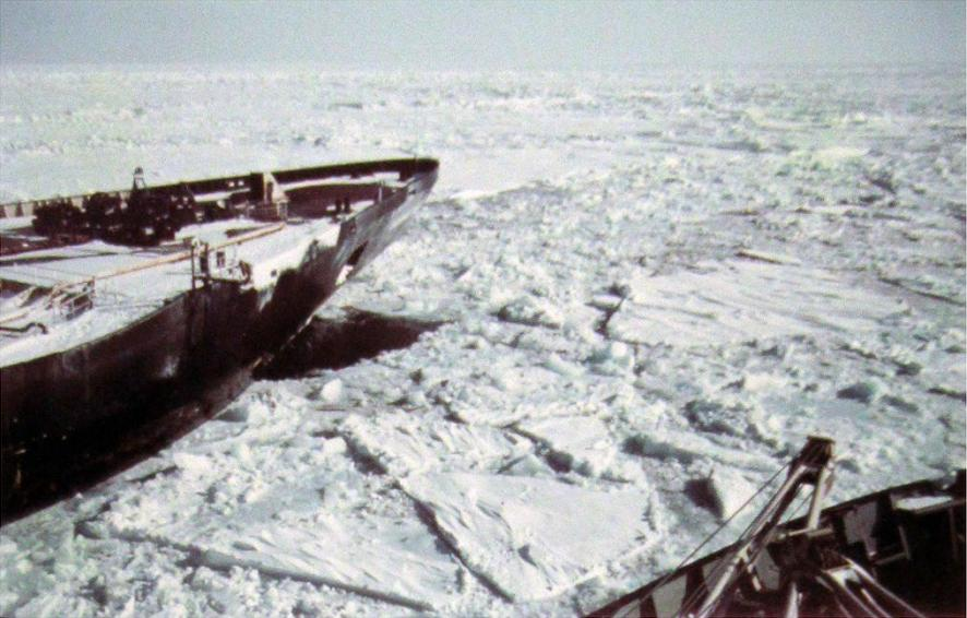
A companion picture to the preceding one. Here the St. Laurent has loosened the ice holding the Manhattan permitting her to back down. Note the size of the broken floes between the two ships and the quantity of debris and brash ice ahead of the tanker. The point where the Manhattan's bow came to rest on her last charge can be seen in the top right corner.
