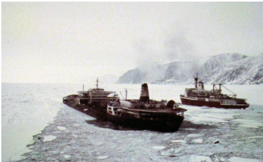
Reference has been made to the problems created by the wide bow of the Manhattan which acted rather like a barb on a fish hook. Once embedded in ice it was difficult to extricate the ship. This picture shows the tanker stuck with ice gripping her around that bow yet with easy conditions apparent from there all the way to the stern.
