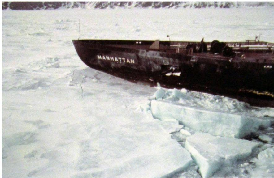
This shows Manhattan breaking some of this Multi-year ice, in this instance it is 8 feet thick. A thin crack can be seen at the stem of the ship running towards the icebreaker from which the picture was taken. Beyond the tanker can be discerned the boundary of this area of heavy ice, beyond which is the smoother, easier, First-year ice through which both ships should have travelled in the first place.
