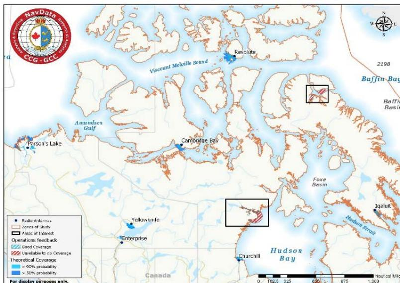
Arctic VHF Radio Coverage Channel 16 - 156.8 MHz
